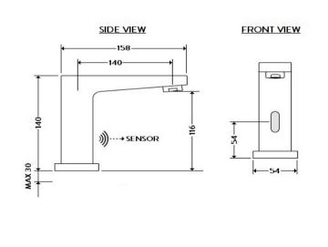
Box contents: INFRA-RED BASIN TAP, CONTROL BOX, POWER ADAPTER, 1X BASE PLATE, 1X 1/2"NUT X 600MM FLEXI PIPE, \*BATTERIES NOT SUPPLIED\*
